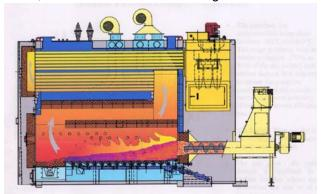
with 45 per cent moisture content. It is warranted at over 80 per cent efficient over its full output range. Fuel is fed to the boiler via augers from the Econergy-designed roll-on roll-off 'hooklift' bin
