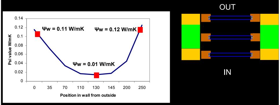
Schematic for illustration purposes based on installation positions for a high performance double glazed window into advanced specification cavity wall construction From "Stamford Brook – making sustainability work" Lowe et al
