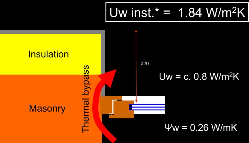
Schematic drawing based on an example from proceedings of the Passive House Conference 2006 for renovation of typical German construction using PH standard window. Freundorfer, Kaufmann and Krause
